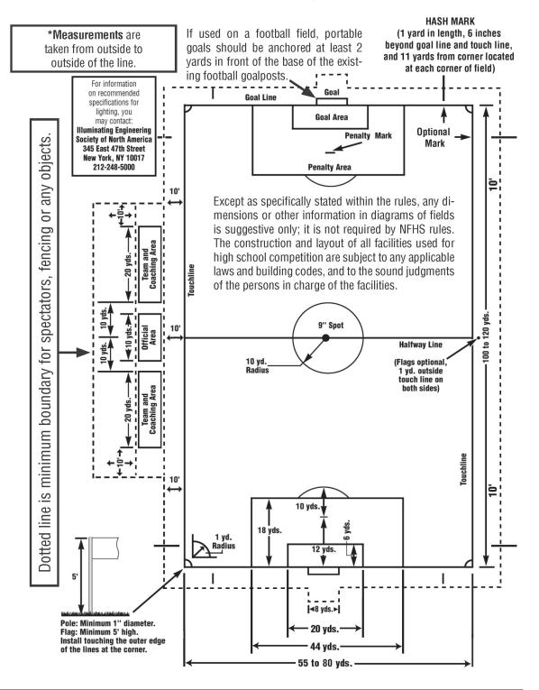
**NOTE:** An engineered natural turf soccer field should have a minimum of one-and-onehalf percent (1.5%) slope for fields which are surface drained. For natural turf fields with a sub-surface drain system the slope should be no less than one (1.0%) percent. For synthetic turf fields with a sub-surface drain system the slope should be no less than one half of one (0.5%) percent. Slope is measured from center to side. For consulting services, contact Design Architects, 816-842-5200.
